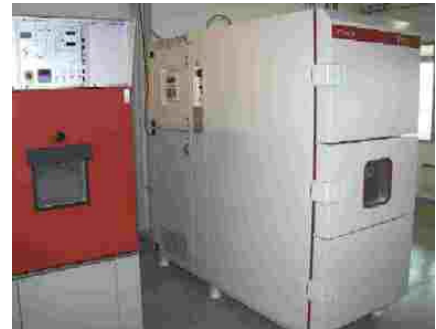
Flux facilities for burn-in and thermal shocks
